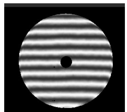
Interferogram of lambda/12 mirror with central hole.
